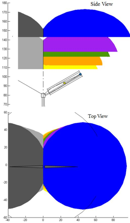
Figure 2. Calculated lightning exposure zones for the Vestas V-90 turbine at an angle of 60 degrees at 8 kA
