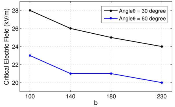
Figure 8. Calculated critical electric field changes for different values of the parameter  $b$
