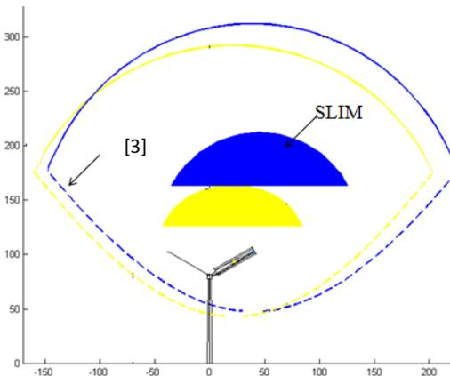
Figure 3. Comparison of the lightning attraction zones estimated by SLIM and the collective volume used in [3] for the tip and inner most receptor (separated by 25 m) at a blade angle of 60 degrees and a prospective return stroke peak current of 15 kA
