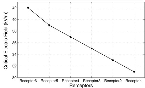
Figure 4. Critical electric field  $E_{stab}$  of self-initiated upward positive lightning for different receptors for the blade angle equal to 60 degrees
