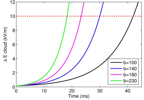
Figure 7. Different rates of change of the thundercloud electric field according to different  $b$  value in equation 2
