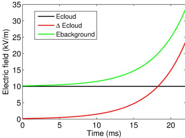
Figure 1. Example of the background electric field under a nearby-lightning triggered flash.
