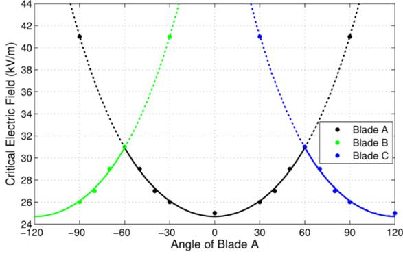
Figure 5. Critical electric field  $E_{stab}$  for the tip receptors on the blades when blade A rotates the upper surface.
