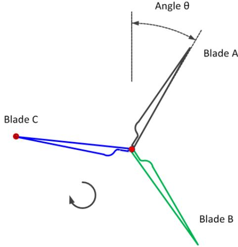
Figure 6. Illustration of the blades and angle  $\theta$
