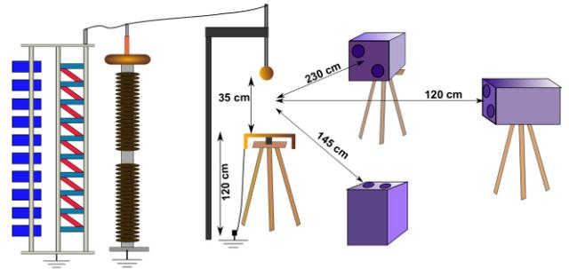
Figure 2. Experimental setup, vertical gap.
