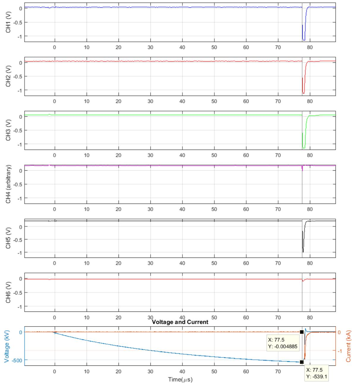
Figure 3. X-rays signals from 6 detectors placed in 3 boxes together with measured voltage and current waveforms.
