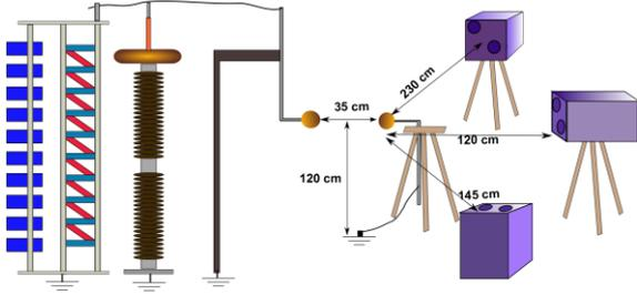
Figure 1. Experimental setup, horizontal gap.
