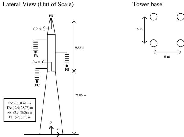
Figure 1. Tower configuration for 138 kV system.
