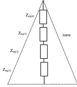
Figure 4. Tower model in ATP.
