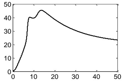
Figure 3. Current waveform obtained from Heidler functions for representation of the first return current (median) measured on the Morro do Cachimbo Station.
