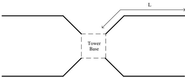
Figure 2. Tower grounding configuration.
