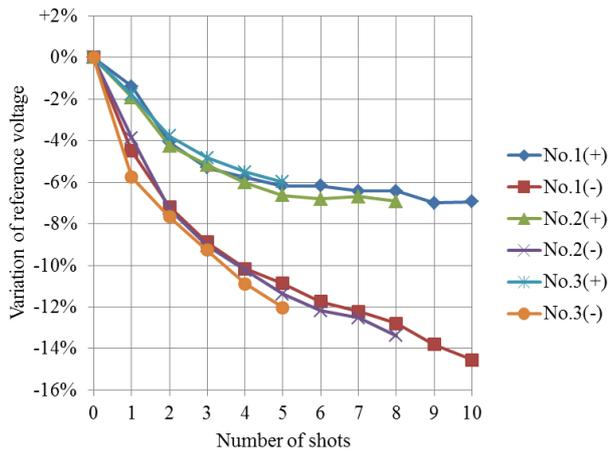
Figure 11. Variation of reference voltage with the impulse current of 100kA (70A/mm<sup>2</sup>)
