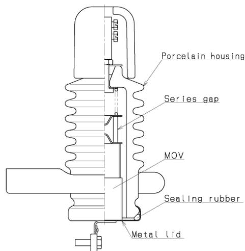
Figure 1. Structure of lightning surge arrester
