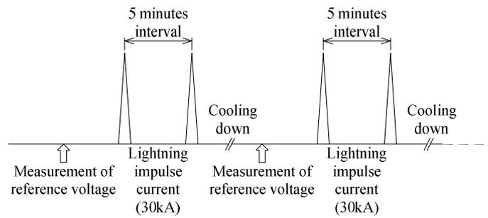
Figure 4. Test procedure of applying lightning impulse currents of 30kA (Test A)
