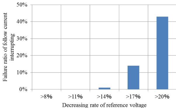
Figure 12. Relationship between decreasing rate of reference voltage of MOV and follow current interrupting failure count
