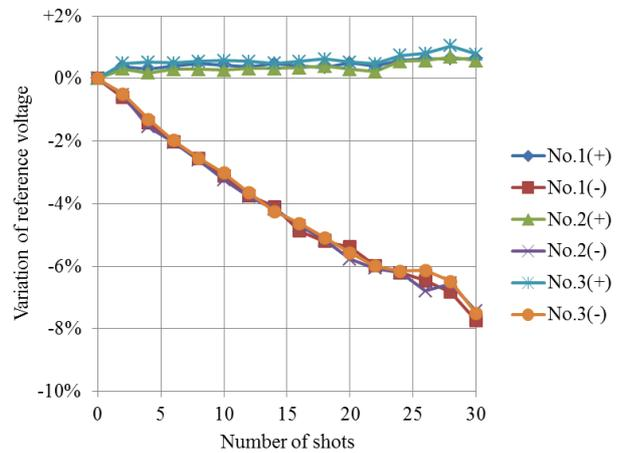
Figure 10. Variation of a reference voltage with the impulse current of 30kA ( 37A/mm<sup>2</sup> )
