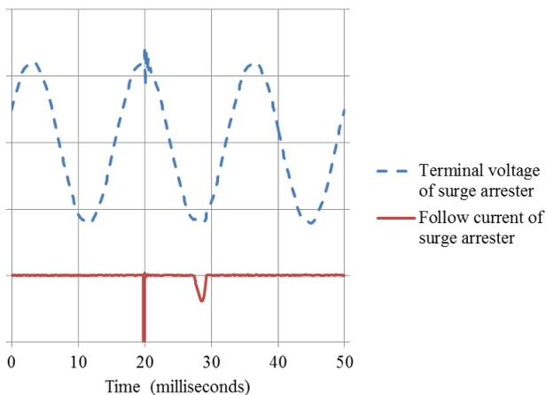
Figure 13. Waveform of follow current interrupting failure
