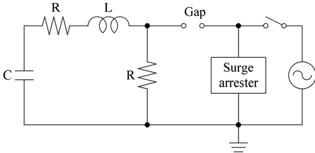
Figure 9. Test circuit of operation duty test (Test C)
