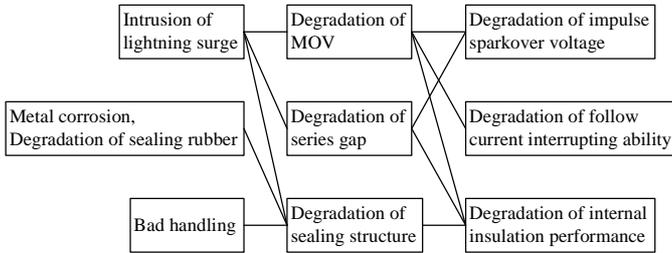
Figure 3. Flowchart of electrical degradation for a gapped surge arrester
