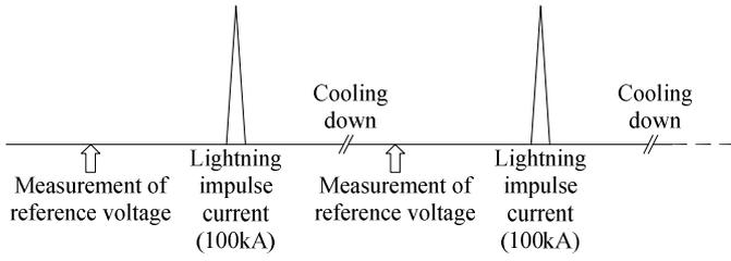
Figure 7. Test procedure of applying lightning impulse currents of 100kA (Test B)
