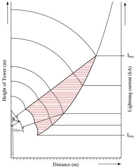
Figure 4. Interception zones of the electrogeometric model
