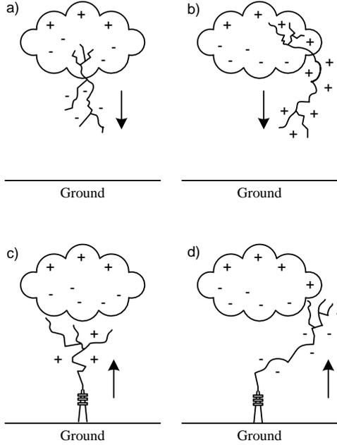
**Figure 2.** Types of lightning discharges a) Downward negative lightning; b) Downward positive lightning; c) Upward positive lightning; d) Upward negative lightning
