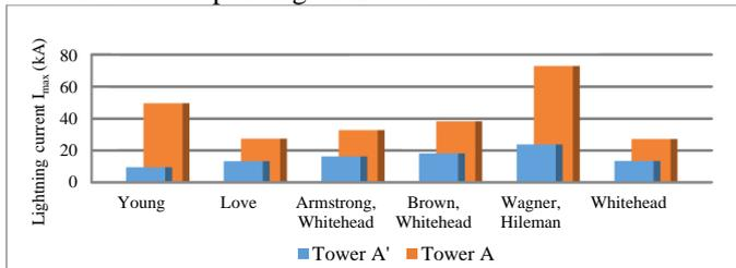
Figure 8. Maximum crest value of the current of a direct lightning stroke to uppermost phase conductor.
