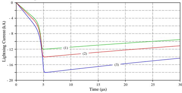
Figure 7. Lightning Current (1) 12 kA; (2) 14 kA ; (3) 18 kA
