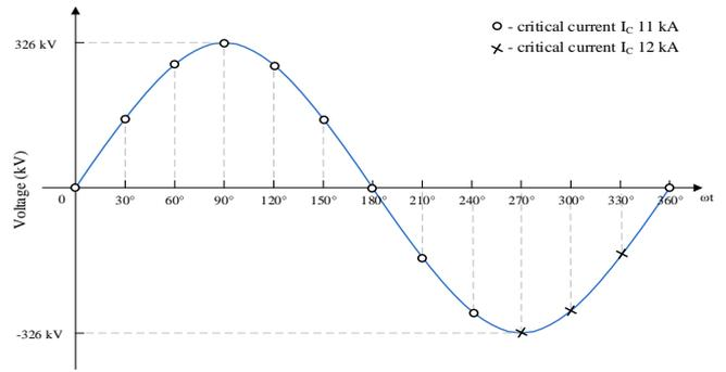
Figure 9. Critical current (380 kV AC System) for each of twelve 30° steps of phase angle
