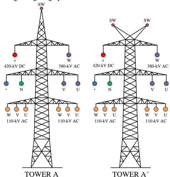
Figure 1. Tower layout of investigated hybrid line A and A'
