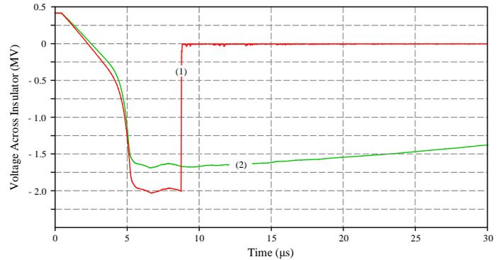
Figure 10. Voltage difference across the insulator string of plus pole causing (1) flashover and (2) no flashover due to shielding failure
