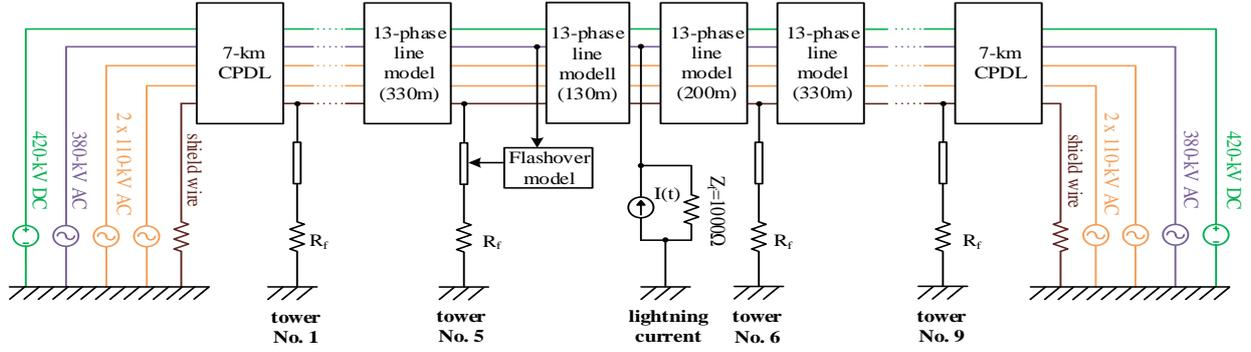
Figure 5. Simulation model for determination of the critical current due to direct lightning stroke
