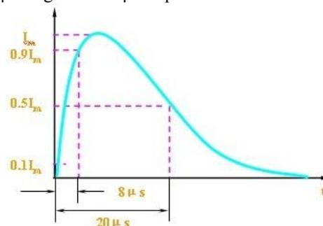
Fig.1 8/20 $\mu$ s impulse current waveform
