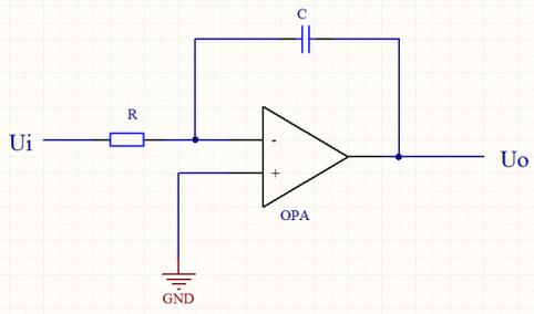
Fig.5 Basic circuit of active integrator
