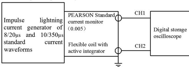
Fig.7 Wiring diagram of current monitoring
