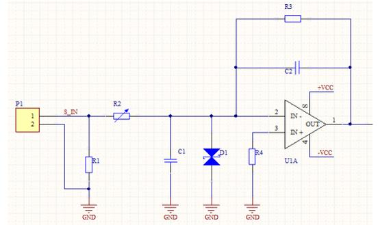
Fig.6 The experimental circuit of practical active integrator
