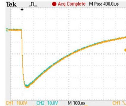
Fig.2 Experimental waveforms of rigid Rogowski coil
