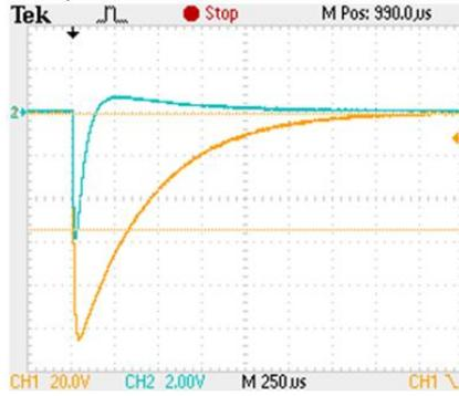
Fig.3 Testing waveforms of flexible Rogowski coil with passive integrator
