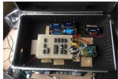
Figure 5 Measurement device for the lightning earth current
