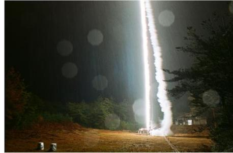
Figure 11 Photograph of the rocket-triggered lightning flash
