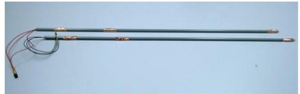
Figure 8 Electrodes for measurement of the lightning earth current
