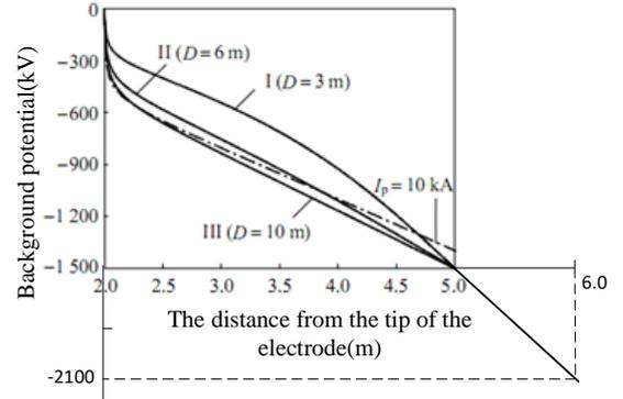
Figure 7. Potential distributions at the axis of inverted rod to plane gaps just before the final jump with different radiuses of upper planes<sup>[13]</sup>
