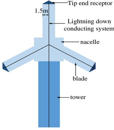
(b) The structure schematic diagram of wind turbine
