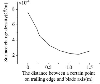
Figure 2. Distribution of charge density at the trailing edge of the blade
