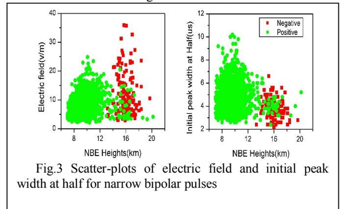
Fig.3 Scatter-plots of electric field and initial peak width at half for narrow bipolar pulses
