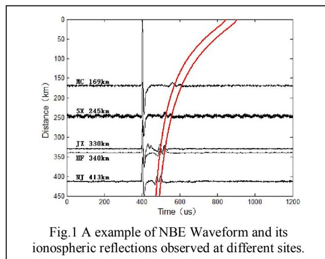
Fig.1 A example of NBE Waveform and its ionospheric reflections observed at different sites.
