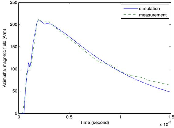
Figure 3. A comparison between the magnetic field simulation and measurement at distance of tower axis, 20 m.
