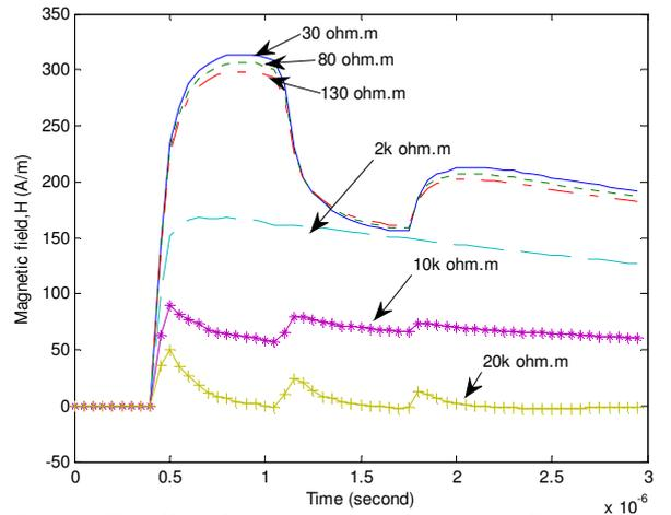
Figure 4. The effect of soil resistivity on the magnetic field wave shape ( $h=100$ m,  $z_0=10$ m,  $r=20$  m,  $t_f=0.15$   $\mu$ s)
