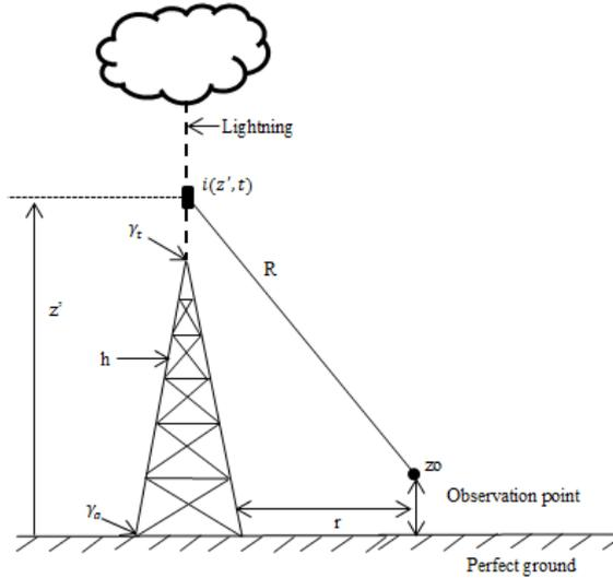
Figure 2. Geometry for the calculation of the magnetic field with respect to a lightning strike on a tower
