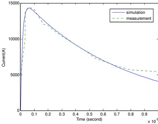
Figure 1. A comparison between the BG function and the measured channel base current at the top of Gaisberg tower, 100 m.
