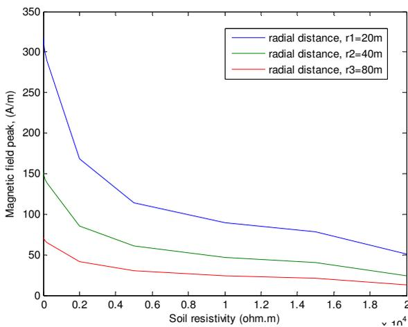
Figure 5. The effect of soil resistivity on the magnetic field peak for different radial distances from the tower struck by lightning ( $h=100\text{m}$ ,  $z_0=10\text{m}$ ,  $t_f=0.15\ \mu\text{s}$ )
