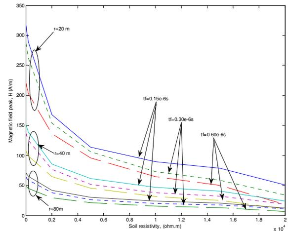
Figure 6. The effect of changes in soil resistivity on the magnetic field peak for different radial distances and front times ( $h=100\text{ m}$ ,  $z_0=10\text{ m}$ )
