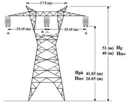
Figure 3. Tower configuration (values in brackets are midspan heights)
