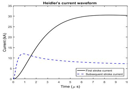
Figure 1. Lightning current waveform
