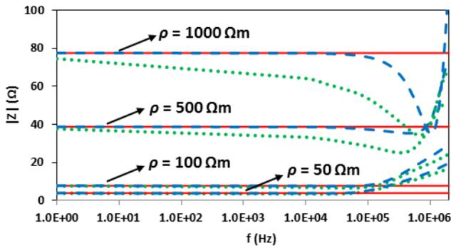
Figure 5. Self-impedances of the vertical rod for different soil resistivities. Red-solid line: simple resistor equal to the dc resistance, blue-dashed line: soil with constant electrical parameters, green-dotted line: soil with frequency-dependent electrical parameters. Adapted from [9].
