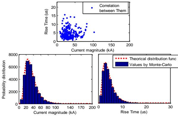
Figure 4. Distribution of randomly generated values of lightning current amplitude and front time with their statistical correlation.
