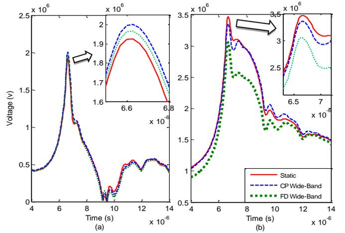
Figure 6. Overvoltages across insulator string in Rod-shape grounding system. Return stroke (100 kA/3.83  $\mu\text{s}$ /75  $\mu\text{s}$ ) (a)  $\rho=100 \Omega\text{m}$ , (b)  $\rho=1000 \Omega\text{m}$ .
