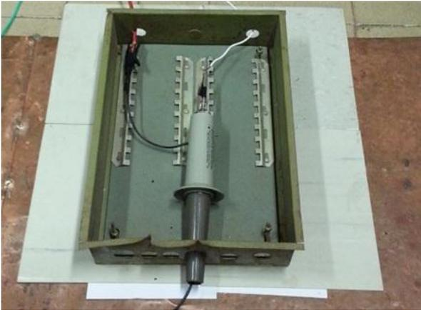
Figure 7. Electrical panel box on the floor, over insulated tiles and paper sheets.
