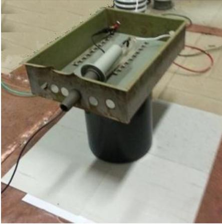
Figure 6. Electrical panel box over an insulator.
