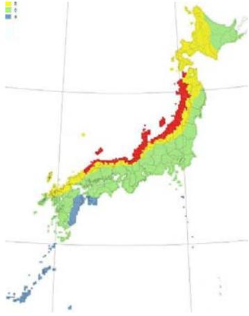
Figure 4. Risk map of high-energy lightning for 120-m wind turbines [10].
