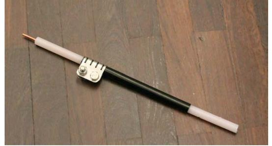
Figure 5. Primed test sample with insulation defect
