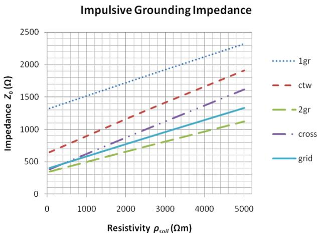
Figure 11. Impulsive grounding impedance  $Z_0$  x resistivity (conventional grounding).
