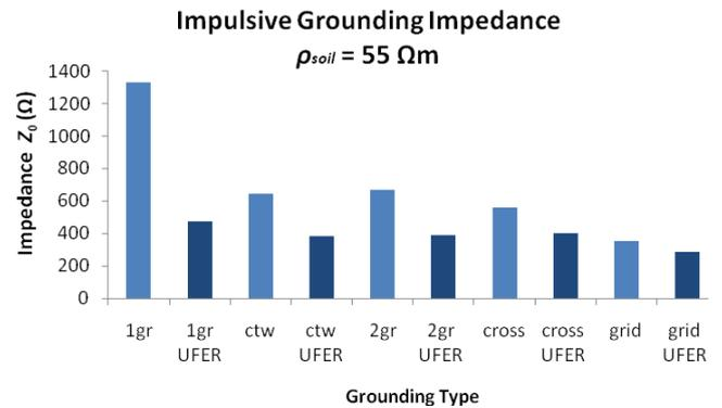
Figure 9. Comparison of different impulsive grounding impedance  $\rho_{soil} = 55 \Omega\text{m}$ .
