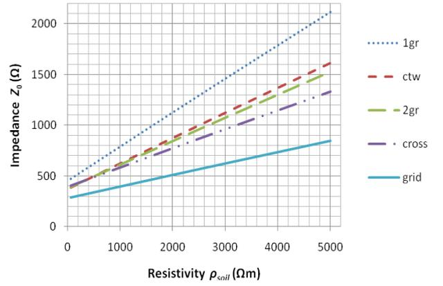
Figure 12. Impulsive grounding impedance  $Z_0$  x resistivity (UFER grounding).
