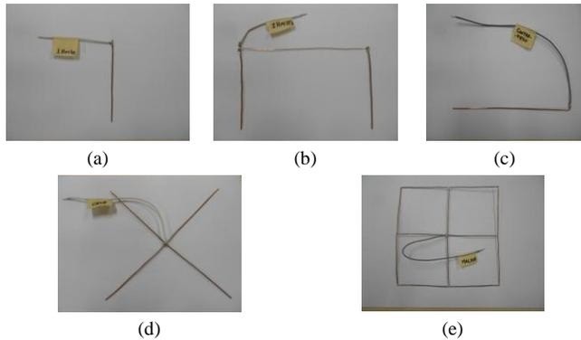
Figure 1. Different types of grounding in reduced scale: (a) 1gr, (b) 2gr, (c) ctw, (d) cross and (e) grid.
