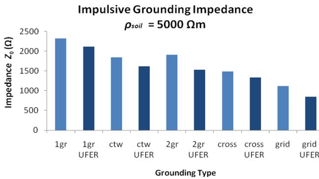
Figure 10. Comparison of different impulsive grounding impedance  $\rho_{soil} = 5000 \Omega m$ .
