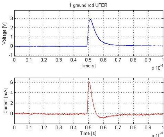
Figure 8. Waveform obtained from grounding 1gr UFER type for a soil with  $\rho_{soil} = 55 \Omega\text{m}$  ( $V_{Max} = 2.90 \text{ V}$ ,  $I_{Max} = 6.10 \text{ mA}$ ,  $Z_0 = 474.79 \Omega$ ).
