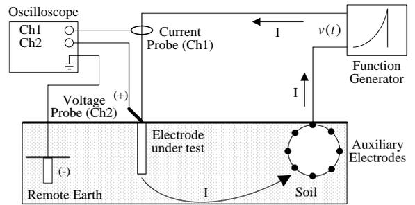
Figure 3. Measuring circuit and the equipment. Adapted from [11].
