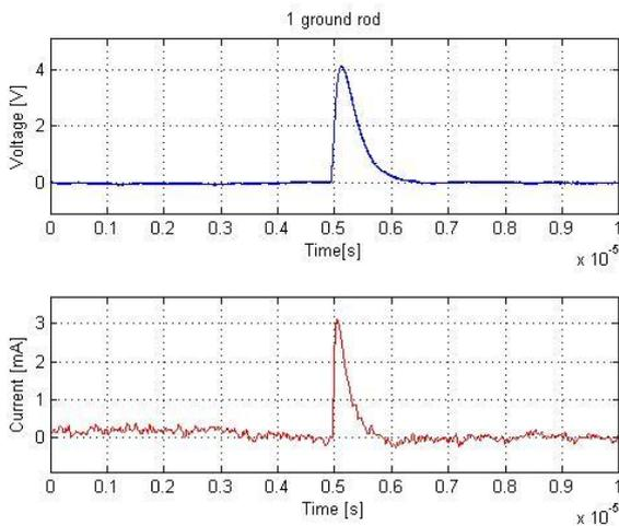
Figure 7. Waveform obtained from grounding 1gr type for a soil with  $\rho_{soil} = 55 \Omega\text{m}$  ( $V_{Max} = 4.14 \text{ V}$ ,  $I_{Max} = 3.11 \text{ mA}$ ,  $Z_0 = 1327 \Omega$ ).
