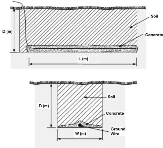
Figure 5. Horizontal installation.
