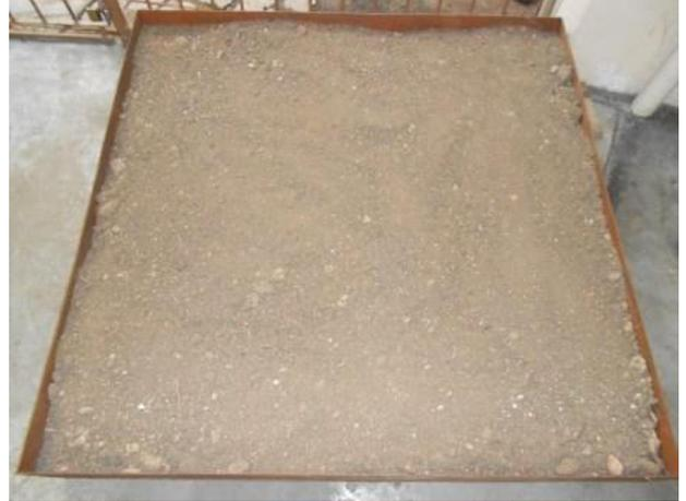
Figure 2. Metal tank with natural earth used in reduced-scale tests.
