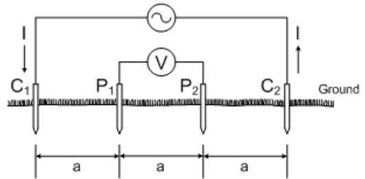
Figure 4. Wenner's Four Electrode Method.
