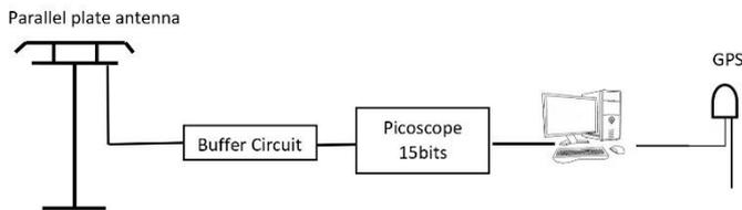
Figure 1. Schematic description of the fast electric field broadband antenna system.
