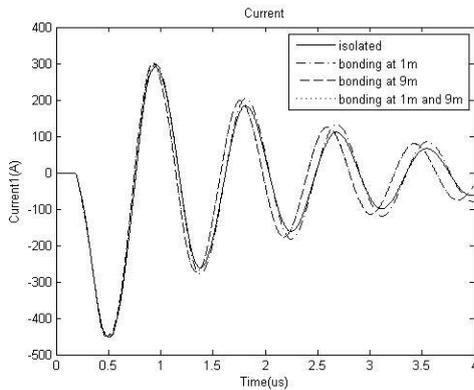
Fig.8. Waveforms of the current in a signal cable with different bonding measures
