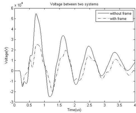
Fig.13. Waveforms of the voltage on the equipment with and without the building frame
