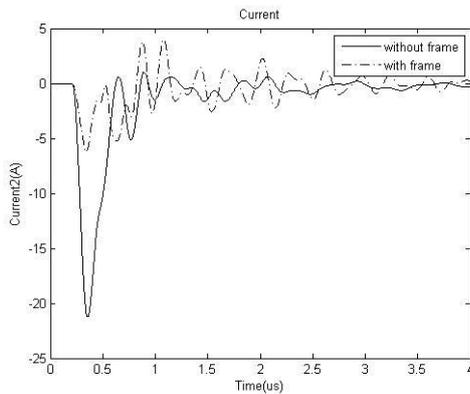
Fig.12. . Waveforms of the current in the protective conductor with and without the building frame
