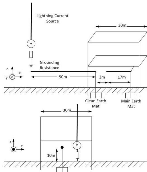
Fig.4. Configuration of the signaling circuit in a building
