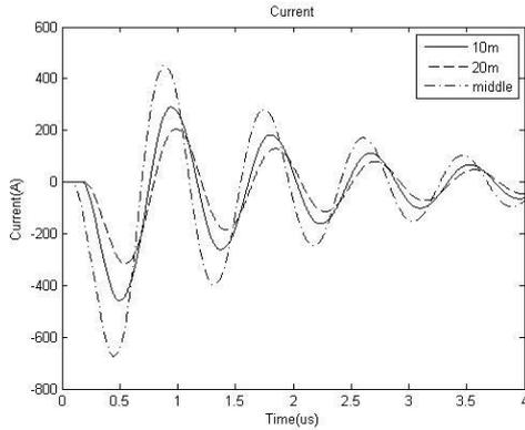
Fig.5. Waveforms of the current in the signal cable with different source positions
