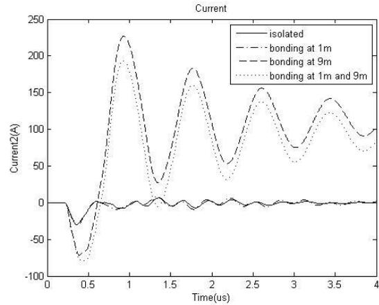
Fig.9. Waveforms of the current in the protective conductor with different bonding measures
