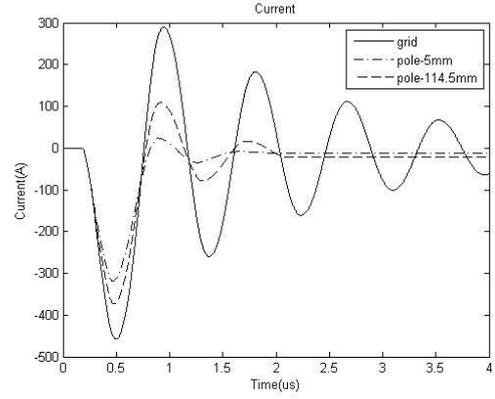
Fig.6. Waveforms of the current in the signal cable with different earthing methods
