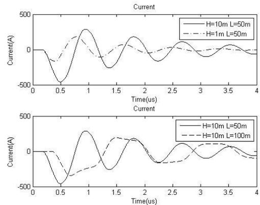
Fig.7. Waveforms of the current in the signal cable with different heights and lengths
