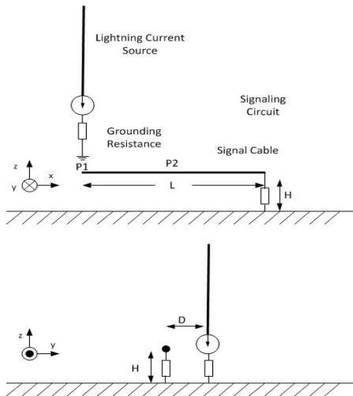
Fig.2. Configuration of the signaling circuit and lightning models
