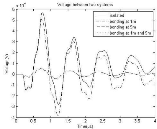
Fig.10. Waveforms of the voltage on the equipment with different bonding measures
