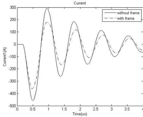
Fig.11. Waveforms of the current in the signal circuit with and without the building frame
