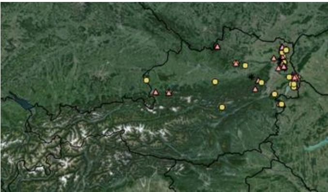
Fig.4: Lightning activity on 2012-02-15 within the border of Austria. Individual strokes are shown as yellow dots (negative CGs), black stars (positive CGs) and red triangles (IC discharges).
