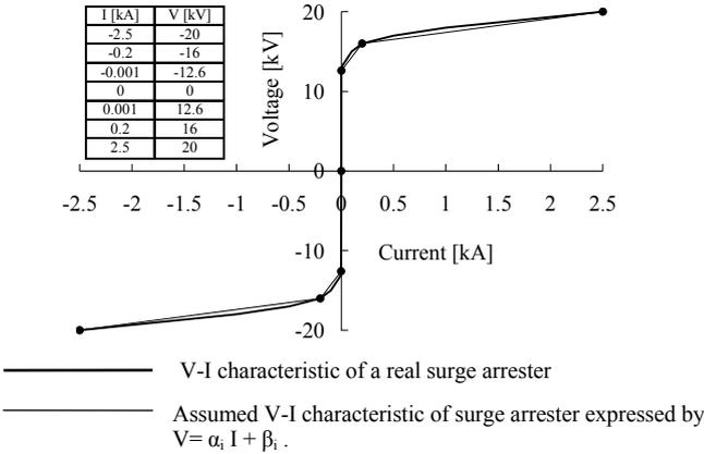
Figure 3. Assumed V-I characteristic of surge arrester passing points in the table.
