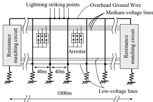
Figure 1. Example of Front view of line subject to analysis
