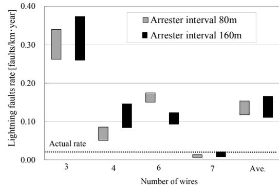
Figure 6. Lightning faults rate for a lightning flash.
