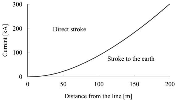
Figure 4. Range of lightning current dependent on the horizontal distance, resulting in direct or indirect stroke to the line.
