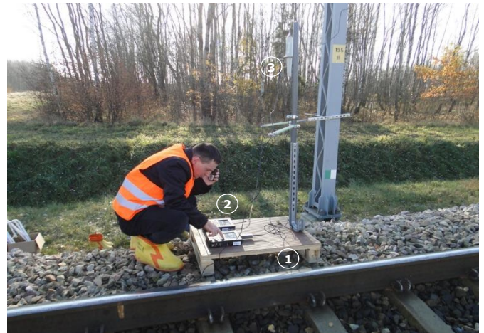
Figure 5. Local measurement post - currents and voltages of SPDs:
