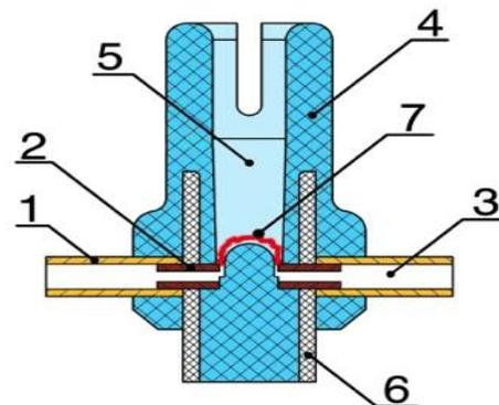
Figure 2. Design of discharge chamber of multi-chamber arrester: 1 – outer tube, 2 – inner tube, 3 – cavity, 4 silicone rubber, 5 – discharge slot, 6 – fiberglass plastic sleeve, 7 – arc.
