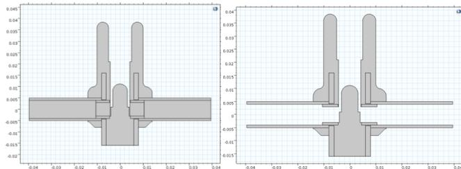
Figure 9. Discharge chamber with solid (left) and hollow (right) electrodes
