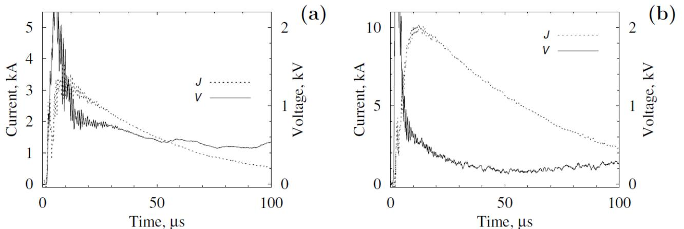
Figure 4. Current (J) and voltage (V) for 10 kA (b) current amplitude test conditions at different time
