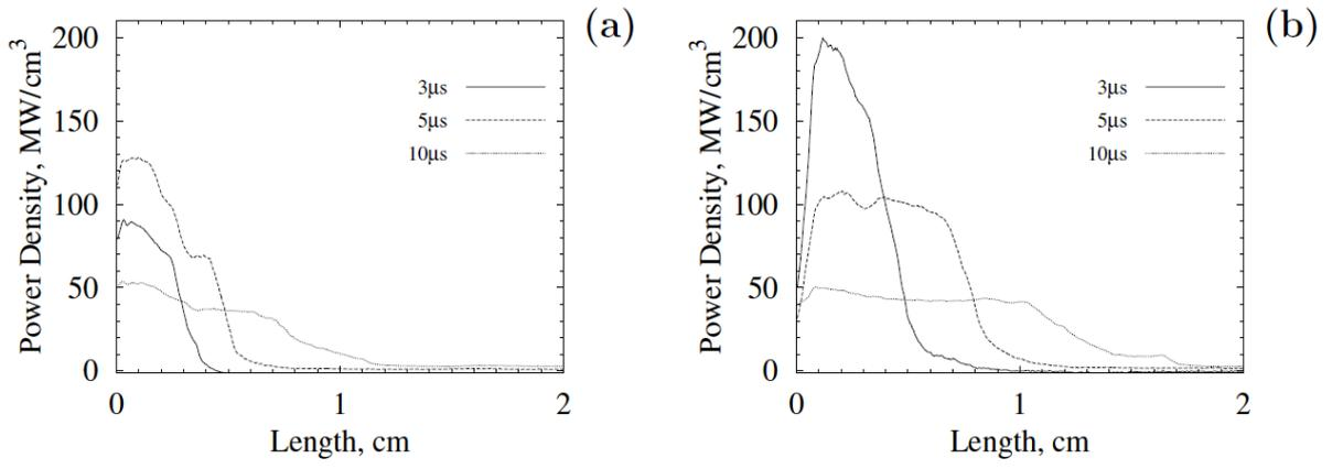
Figure 5. Energy deposition distribution along discharge chamber for 3kA(a) and 10kA(b) current amplitude test conditions at different time
