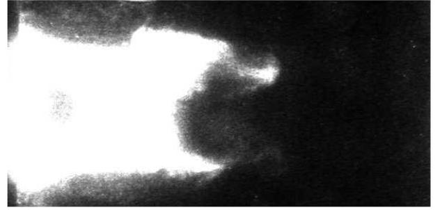
Figure 3. High-speed photo of discharge for current amplitude 10 kA after  $10\mu\text{s}$
