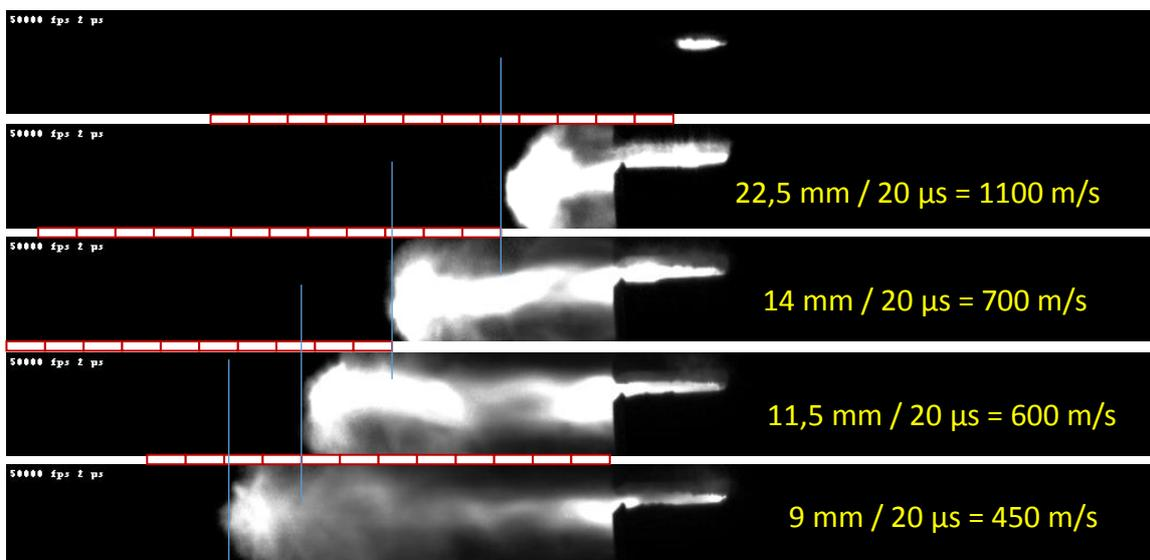
Figure 12. High speed imaging of plasma jet out of discharge chamber
