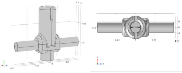
Figure 7. Discharge chamber 3D-model: Left-general view, Right – Top View.
