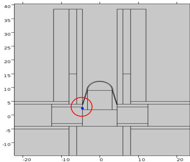
Figure 15. Transition zone (marked by red circle). The depicted blue point is set for velocity calculation
