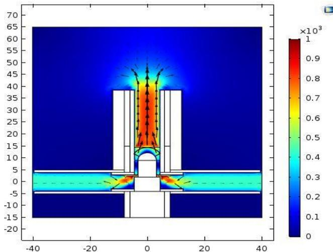
Figure 10. Flow velocity distribution. The units for color bar numbers are m/s
