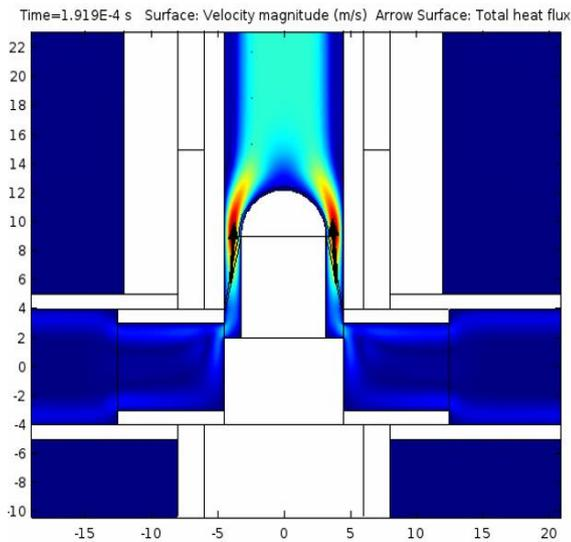
Figure 17. The diagram of flow velocity for  $t=19.2 \mu\text{s}$ . The arrows point to the direction of heat flux. The arrow size is proportional to heat flux magnitude
