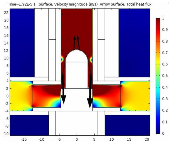
Figure 18. The diagram of flow velocity for  $t=192 \mu\text{s}$ . The arrows point to the direction of heat flux. The arrow size is proportional to heat flux magnitude
