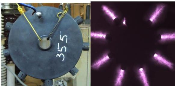
Figure 1. Design of multi-chamber arrester (left) and impulse arc discharge in multi-chamber arrester (right).
