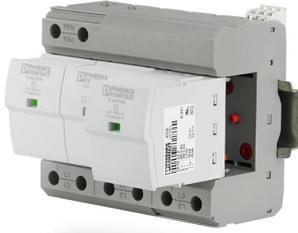
Figure 4. Class I lightning current arrester based on triggered and encapsulated spark-gap technology for the protection of a three phase TN-C-system (FLT-SEC-P-T1-3C-350/25-FM) [7].
