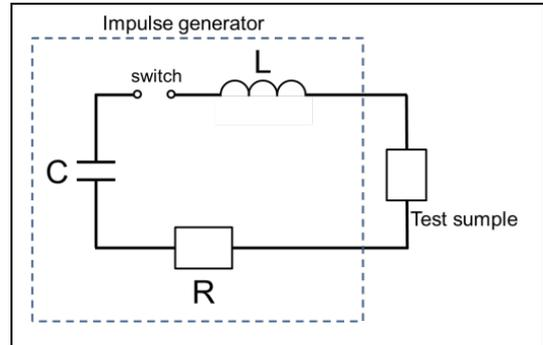
Fig.6 Impulse generator (test circuit)
