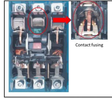
Fig. 3 Example of circuit breaker failure in short circuit mode
