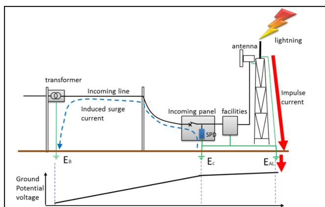
Fig.1 Surge current to power line due to direct lightning strike
