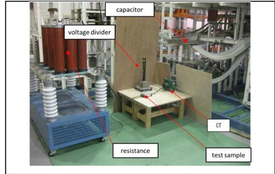
Fig.5 Impulse generator (test setup)
