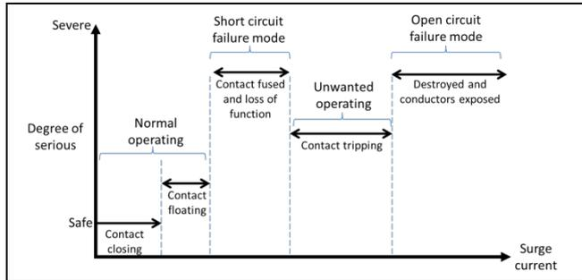
Fig.8 Relationship between impulse current value and circuit breaker failure mode
