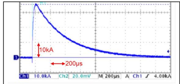
Fig.7 The example of impulse current waveform
