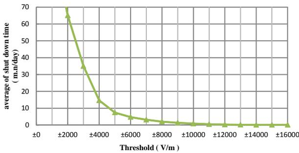
Fig. 8 Threshold – average shutdown time characteristics.
