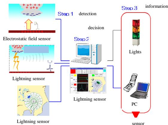
Fig. 1. System configuration diagram.
